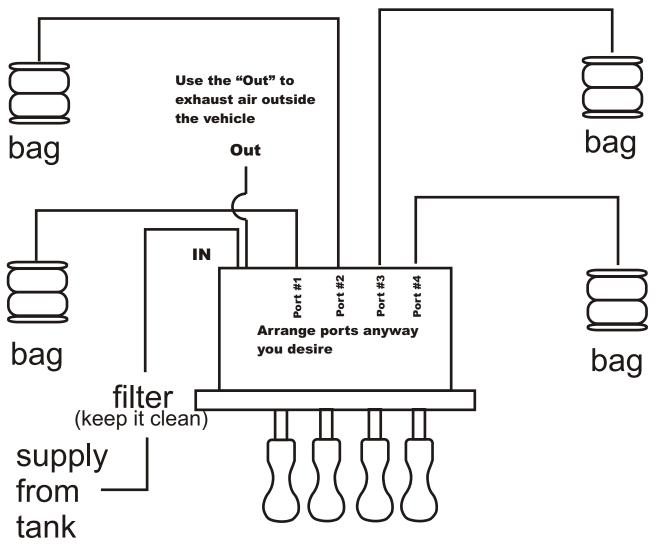
The larger the air lines you use, the faster your bags will fill and drain. Internal valve design will handle 1/2" OD hose. All port connections are 3/8" NPT except the gauge port is 1/8" NPT. Install a filter in your supply line to increase the life of your system. When the valves are new the valves may stick. Use motor oil to lubricate the brass spools that can be seen through the slots behind the handles and about 10 drops in the "IN" port.
